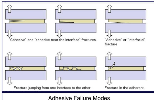
A failure analysis can help determine the location and cause of an adhesive failure, help understand the mechanisms of the crack initiation and propagation, and identify the weakest link in the structure.
