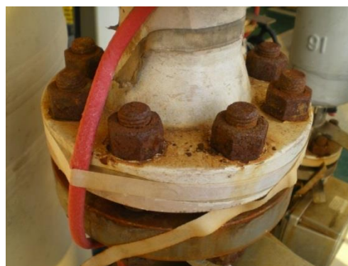
Fig 12 - Bolt corrosion after 18 months offshore North Sea
