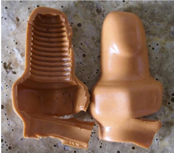
Fig 22 - comparison with a reference sample shows slight colour loss after 4500 hours
