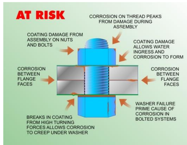
Fig 1 - coating damage during assembly
