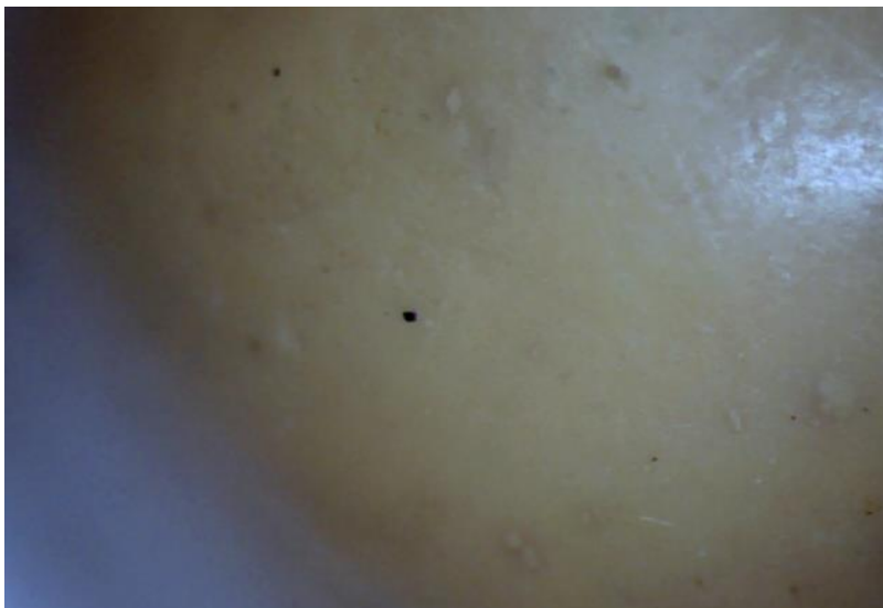
Fig 23 - close examination showed no crazing or cracking of the surface
