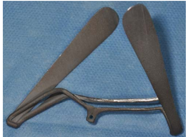
Fig. 7. Manufactured instrument by laser sintering technology.
