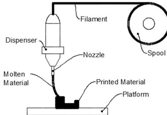
after the extrusion. The nozzle is moved along the horizontal and vertical directions by a numerically controlled mechanism (Bralla & Press, 2007; Miller, Vandome, & McBrewster, 2010). While the material is extruded as a thin ribbon on the work surface, the CAD model can be constructed layer by layer in a computer controlled pattern.
