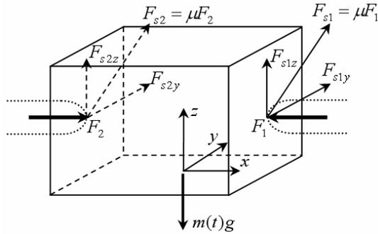
Fig. 3. Representation of forces acting on load.
