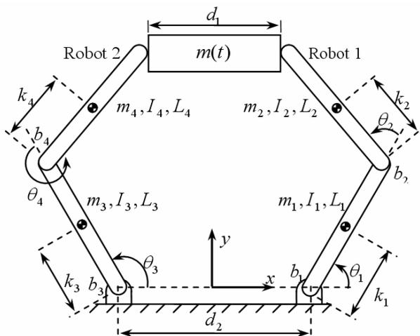
Fig. 1. Physical model of the robot arms.
