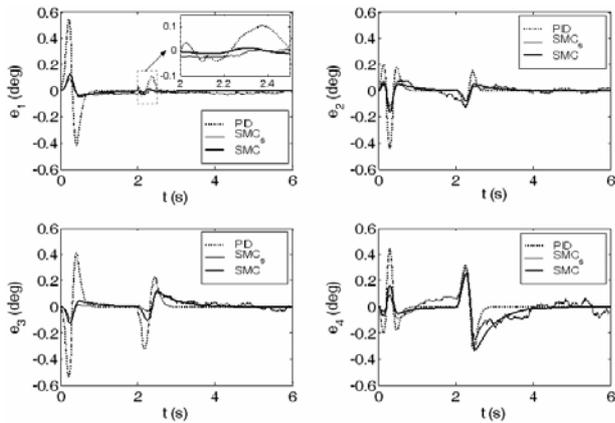
Fig. 8. Tracking errors of the related joint angles.
