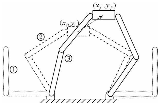
Fig. 2. Motion of the robot arms.
