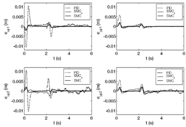
Fig. 9. Tracking errors of the endpoints of the robot arms.
