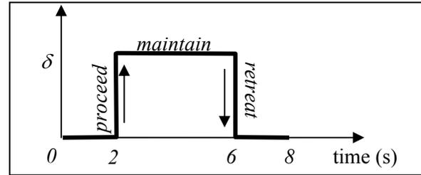
**Figure2.** Displacement – Time profile [12]
