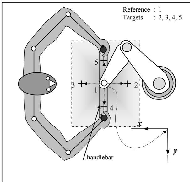
**Figure1.** Experimental set-up for EMG signals measurements [12]
