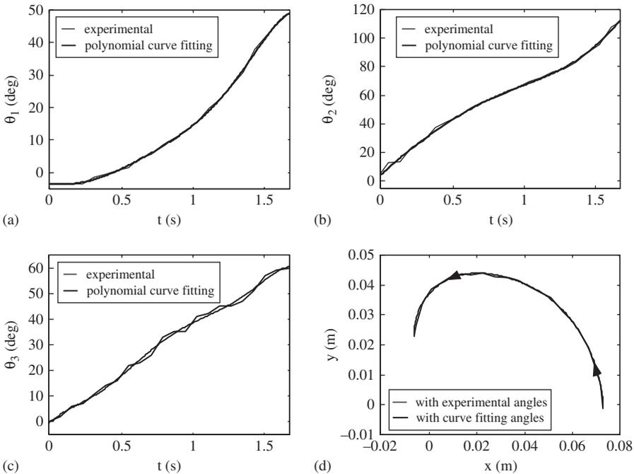
**Figure 7:** (a), (b), (c) Experimental data of joint angles and their polynomial approximations; (d) trajectory of the robot finger for closing motion.
