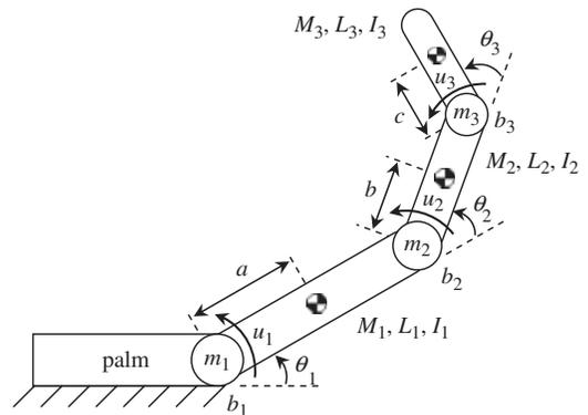
**Figure 2:** *Finger model of the humanoid robot hand.*
