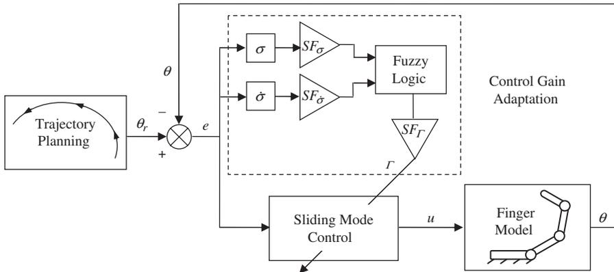
**Figure 6:** The system and controller structure.
