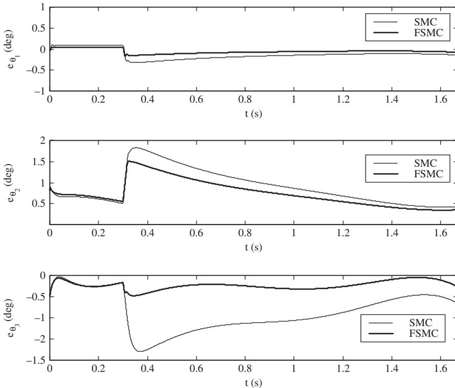
**Figure 11:** Comparison of the related joint angle errors for a conventional sliding mode controller (SMC) and the proposed fuzzy sliding mode controller (FSMC).
