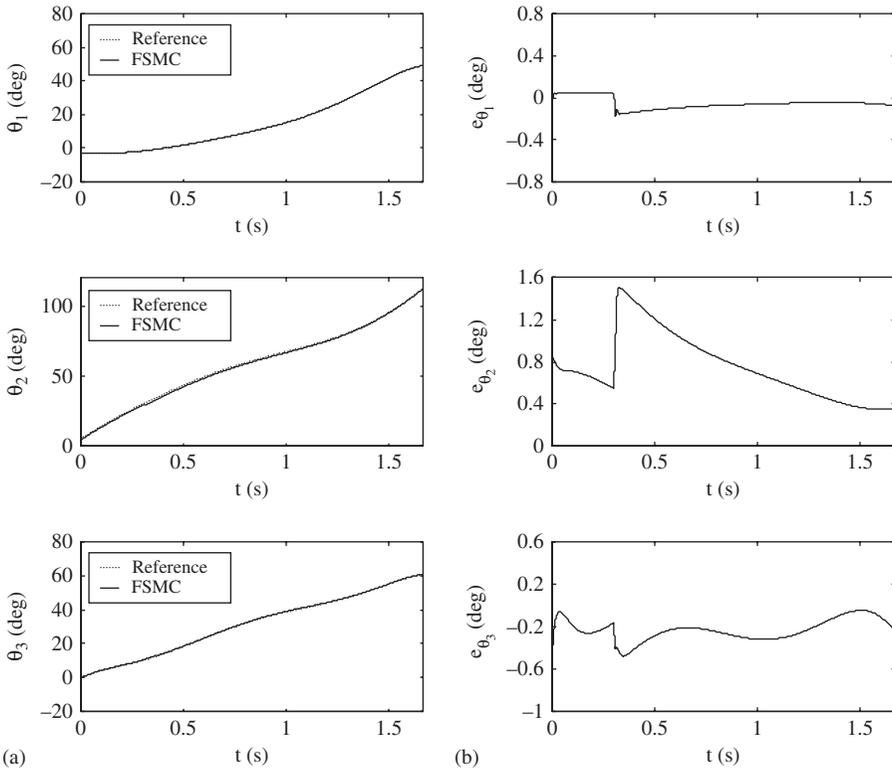
**Figure 9:** (a) Reference and actual values for joint angles; (b) tracking errors for the links.
