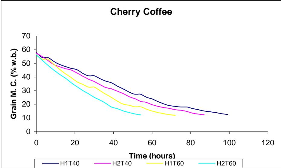
Fig. 3: Drying curve for natural coffee cherry using terrace drying with heated air aeration system – H1 (solar + biomass energy) and H2 (only biomass energy)
