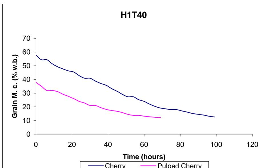
Fig. 5: Drying curves for pulped cherry and for natural coffee cherry using drying terrace with heated air aeration system – H1 (solar + biomass energy)
