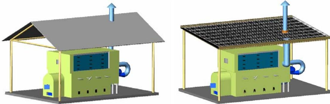
Fig. 6a: Flex dryer with traditional roof      Fig. 6b: Flex dryer with a solar roof collector
