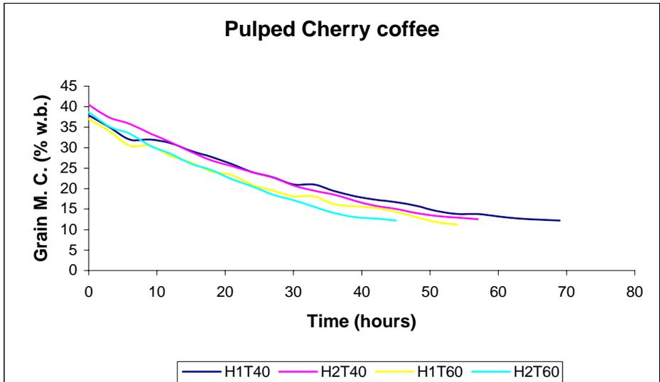
Fig. 4: Drying curve for pulped coffee cherry using terrace drying with heated air aeration system – H1 (solar + biomass energy) and H2 (only biomass energy)
