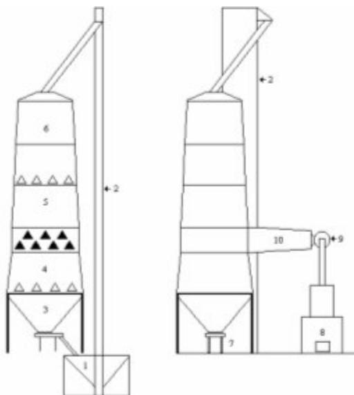
Fig. 8: Details of a drier with mixed flows
