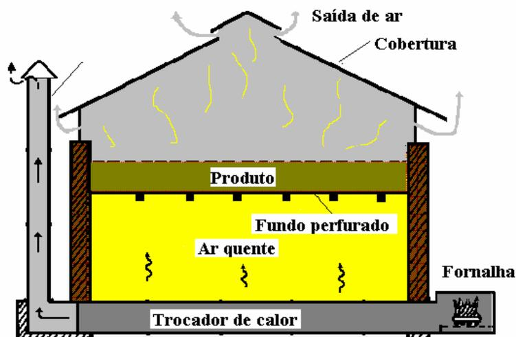
Fig. 7: Longitudinal section of a natural convection dryer
