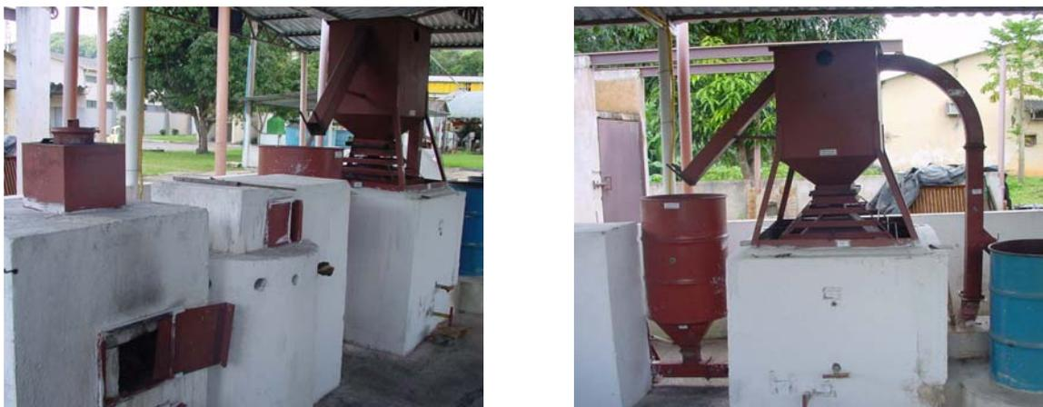
*Fig. 9: On the left showing the furnace and cyclone; on the right the two resting chambers (with the second mounted on the pyramids)*
