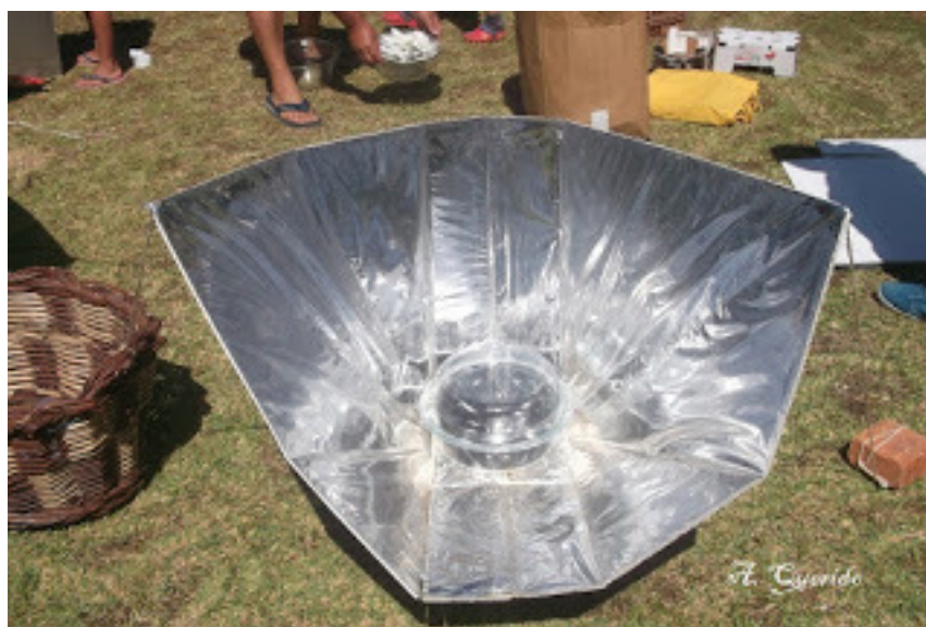
Figure 4. Baking a cake using a solar funnel cooker [12])
