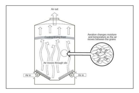
Diagram outlining the cooling/drying fronts occurring in the aeration process of stored grain within silos
