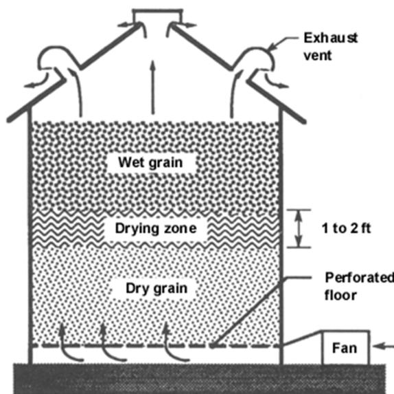
Figure 1. Schematic of natural-air drying bin.
