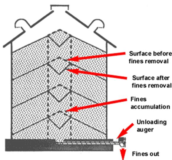
Figure 2. Removing fines during bin filling.
