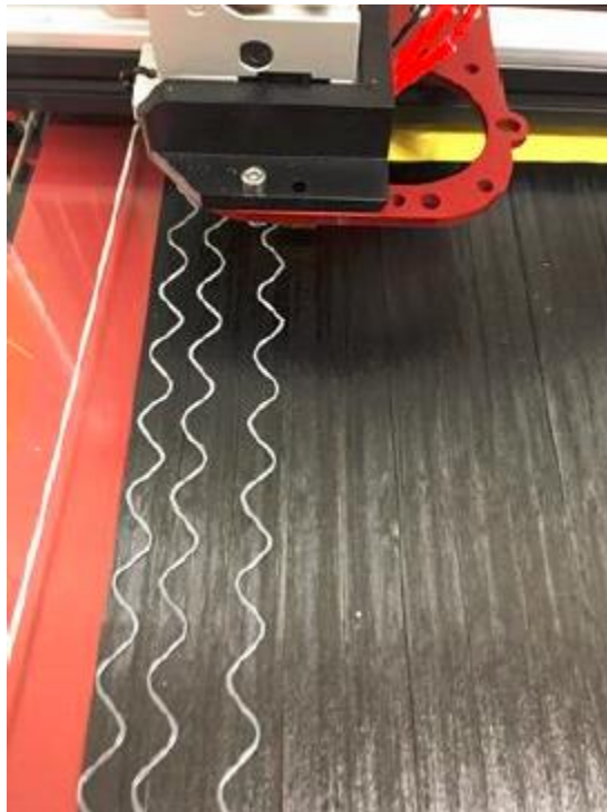
Figure 2: Microchannels being laid out on composite, which will be embedded under further layers [3]
