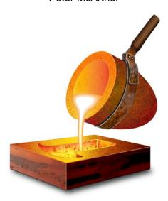
**Moulding** (or **molding** if you're American) is a method of manufacturing to shape a liquid or some pliable raw material using a frame (rigid or rubber) called a mould or matrix. Think of a cake mixture, or a child's plaster of Paris (gypsum plaster) to make a toy figure. Anything really, from a piece of pottery, to a ceiling decoration, or a child's fantasy figure. You know the thing I'm sure; see below.
