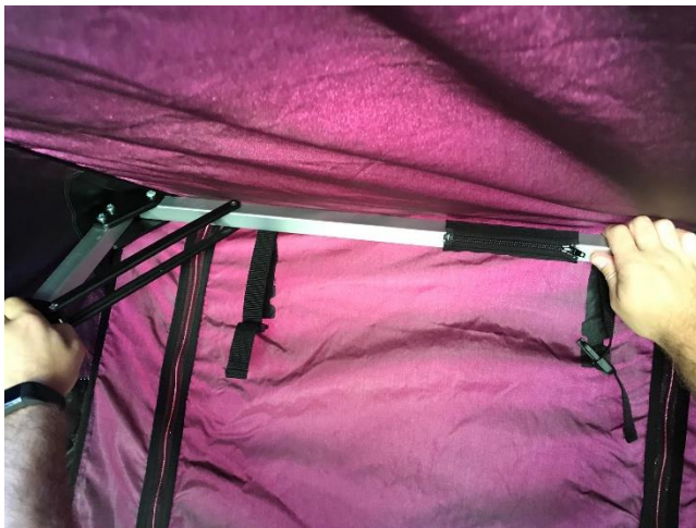
Figure 7.5.1 Disengage Truss System (Left Side)
