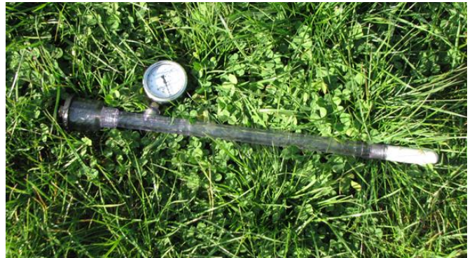
Figure 1. Tensiometer. Typically under pasture the porous ceramic moisture sensor on the end of the tensiometer is buried in the active rootzone at 20cm soil depth.
