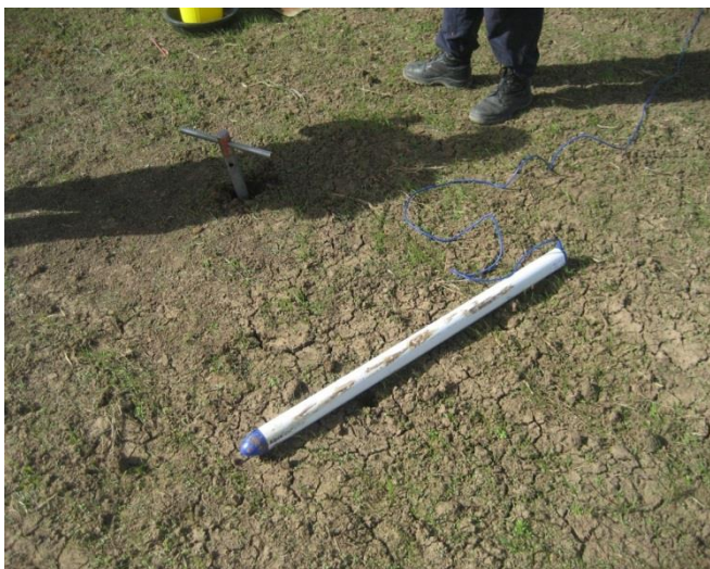
Figure 2. Capacitance probe in the process of being installed. Photo courtesy of Dale Boyd, Agriculture Victoria.
