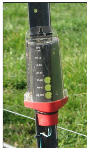
Figure 3. Left: A manual-read visual display unit ("GDot") mounted on a laneway fence-post. It is hard-wired to a gypsum block moisture sensor installed under irrigated pasture. The irrigator views this unit regularly from a passing motor-bike.
