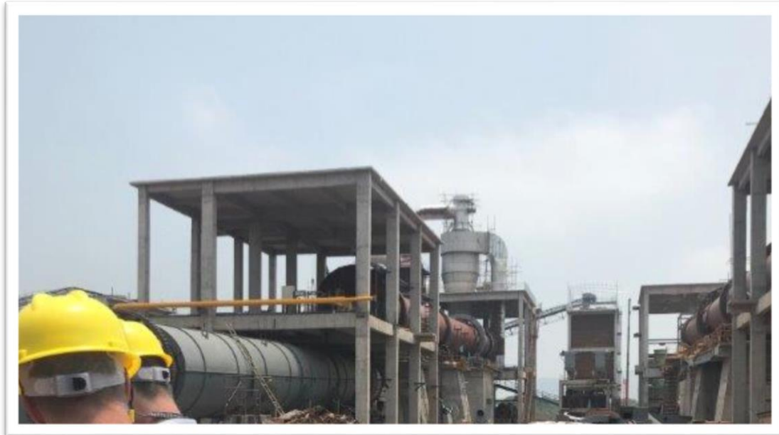
FIGURE 4: ROTARY KILNS USED TO CALCINE LITHIUM MICA WITH SULPHATE PRIOR TO WATER LEACHING
