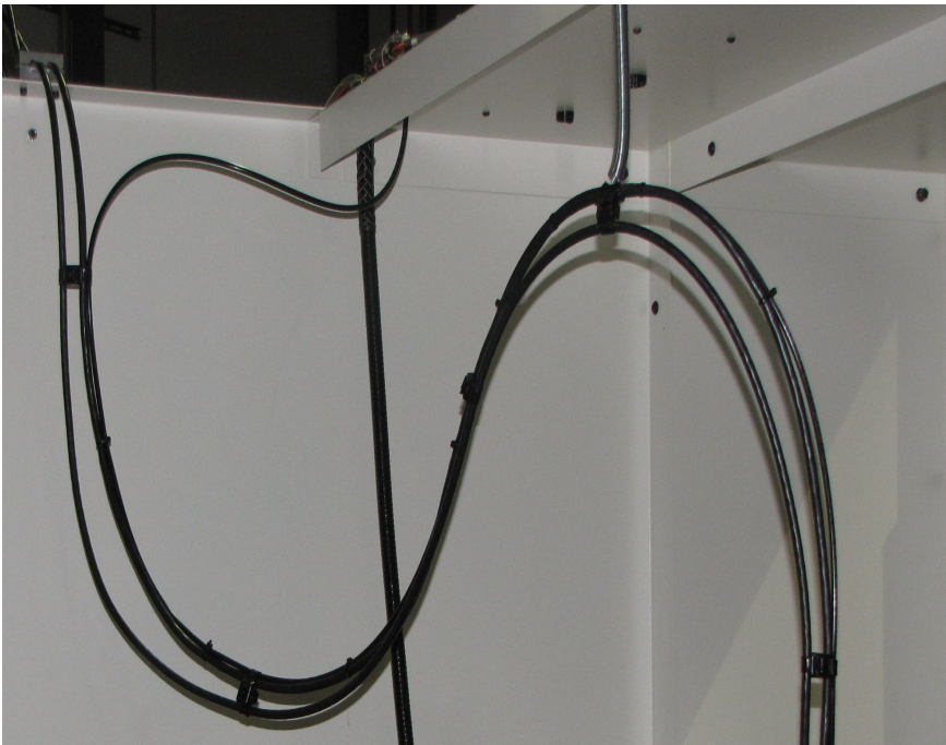
Figure 16, Make sure there is enough slack for machines table to move its complete travel with the rotary tables cables held up and out of the chip trays
