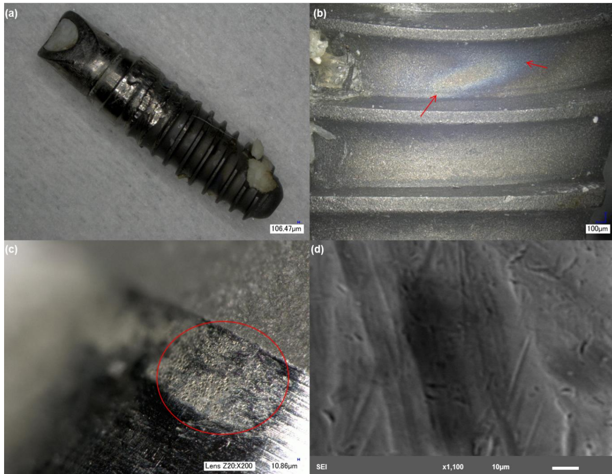
Figure 4. Structure of implant 3. (a) Low magnification showing the gross features of the implant and bone attachment to the bottom part of the surface; (b) discoloration is also evident in this example; (c) severe pitting attack on the top interface of the implant in the abutment region; and (d) higher magnification of an area of the abutment with scratching.
