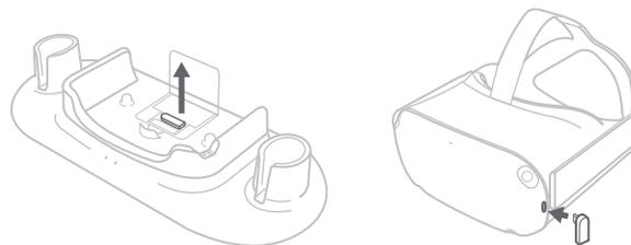
4. Place your Quest™ VR headset to charge. When charging, the LED on your VR headset will turn GREEN. Built-in automatic idle charging control protects your device from overcharging. The LED remains GREEN when it's idle.
