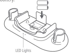
3. When the batteries are charging, the LED is RED; when it's ready to use, the LED is GREEN.
