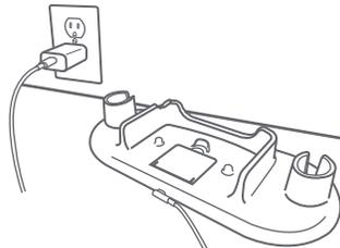
2. Place two AA NiMH rechargeable batteries (not included) into the charging bay. This charger is designed to use with NiMH batteries. Use of other batteries is not supported. 1600-2500mAh battery is recommended for each battery.
