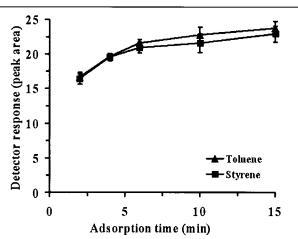
**Figure 4.** Effect of adsorption time on the amount of styrene and toluene detected in serum at a standard concentration of 10 ng/10  $\mu$ L. Values are means of three independent determinations, and error bars indicate standard deviation. Operating parameters: desorption time, 30 s; sample volume, 10  $\mu$ L; desorption fiber depth, 3.7 cm; and adsorption temperature, 23°C.
