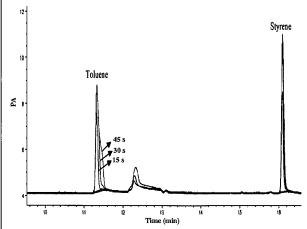
**Figure 2.** Overlaid chromatograms of three runs differing in time of desorption of the fiber.
