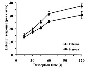
**Figure 1.** Effect of desorption time on the amount of styrene and toluene detected in serum. Values are means of three independent determinations, and error bars indicate standard deviation. Operating parameters: desorption fiber depth, 3.7 cm; sample volume,  $10 \, \mu L$ ; adsorption time, 4 min; and adsorption temperature,  $23 \, ^{\circ}C$ .
