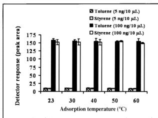
**Figure 5.** Effect of adsorption temperature on amount of styrene and toluene detected in serum at standard concentration levels of 5 and 10 ng/10  $\mu$ L. Values are means of three independent determinations, and error bars indicate standard deviation. Operating parameters: desorption time, 30 s; sample volume, 10  $\mu$ L; desorption fiber depth, 3.7 cm; and adsorption time, 4 min.
