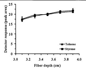
**Figure 3.** Effect of fiber depth in the injection port of the GC during desorption on the amount of styrene and toluene detected in serum. Values are means of three independent determinations, and error bars indicate standard deviation. Operating parameters: desorption time, 30 s; sample volume, 10  $\mu$ L; adsorption time, 4 min; and adsorption temperature, 23°C.
