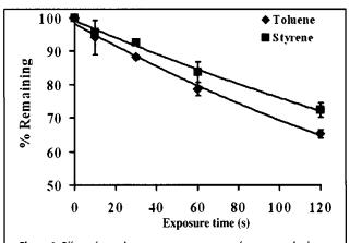
**Figure 9.** Effect of sample exposure on recovery of styrene and toluene. The loss of styrene and toluene in whole blood as a function of time from a 10- $\mu$ L sample was determined at the concentration level of 1 ng/10  $\mu$ L. The 100% reference indicates the amount of styrene and toluene recovered from stock solution before exposing the sample to the atmosphere. Values shown are means of three independent readings, and the error bars indicate standard deviation.
