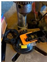
With the hole location template, drill a hole using the supplied drill bit in the back of the door handle unit.
