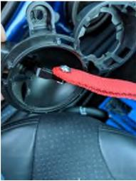
Screw the flanged bolt into the sleeved nut until tight.
