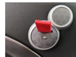
Slide the strap through the cover plate. Place the long Allen bolt through the centre hole and locate the hole previously drilled. Tighten until cover plate is secure (do not over tighten).
