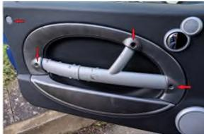
Remove door handle cover reflector cap.
