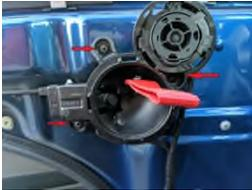
Screw in the screws for the handle housing. Now test the new door pull by closing the door and pulling the strap to open. The Mechanism may catch on the door metal work, use the supplied rubber washers to step the door handle off the door
