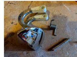
Remove the handle and spring (these are no longer needed, keep in safe place if you wish to reverse the process) Keep the pin as this is required
