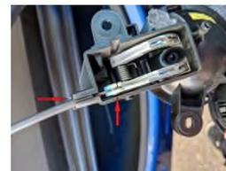
Slide the cable cover back and unclip the cable from the handle mechanism.
