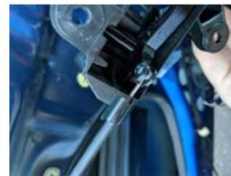
Slide the cable cover back and into the handle housing.
