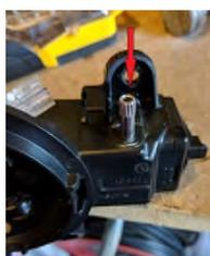
Tap the pin through the unit and mechanism until it is showing on the other side.
