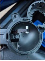
Insert the sleeve nut through the mechanism.
