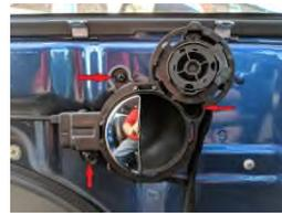
Unscrew the 3 screws holding the handle unit.
