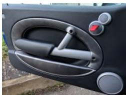
Re-attach all the bolts holding the door card and slide the door handle cover on. Stand back and enjoy your new Door Pull opener.
