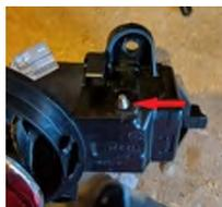
Remove the pin from the unit. A tap with a hammer loosens it then pull out with pliers
