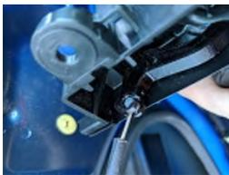
Clip the cable into the mechanism.
