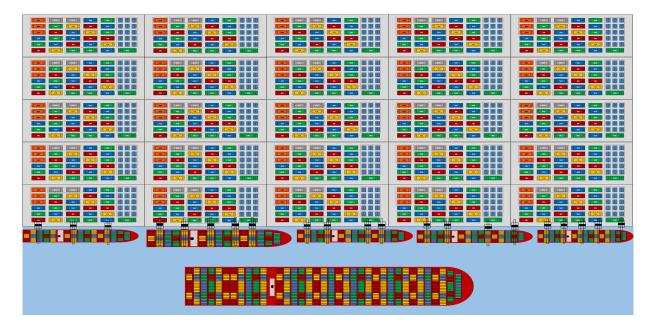
How on earth are you going to operate it? For one, it is going to use a massive amount of your most valuable asset, the quay wall. Secondly, it would not be practical to scale up current gantry cranes to work the vessel because they simply wouldn't support their own weight and, because they would have to increase in width, you will lose productivity because you may need 2-3 bays between each crane.
