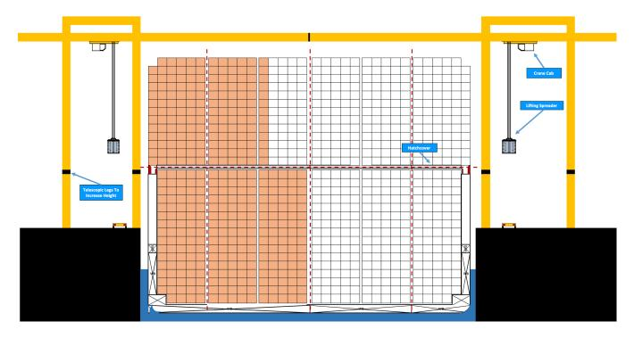
If we then design a system where the crane boom can retract, as opposed to lifting the boom up, not only do we solve the issue of having massively over-engineered gantry cranes but we can now work many more bays simultaneously and we can work from both sides of the vessel.
