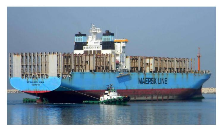
The concept was brilliant.....on paper. The reality was that the unsupported cell guides that can be see above the hull were very prone to damage during cargo operations which meant that, as the vessels got older, the problems increased. This concept has been largely abandoned today.
