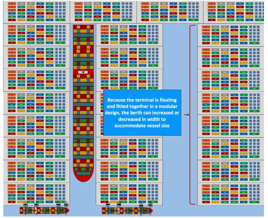
The berth size was not the only limiting factor for this terminal. Its designers failed to look at the landside infrastructure. There were limited options for moving cargo inland and so the shippers stayed away.
