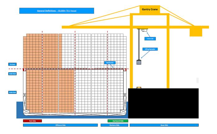
As can easily be seen, with current crane designs, the shaded are of the vessel is now inaccessible to the crane. There is always the option of turning the vessel around during operations but this is time consuming, costly and potentially risky.
