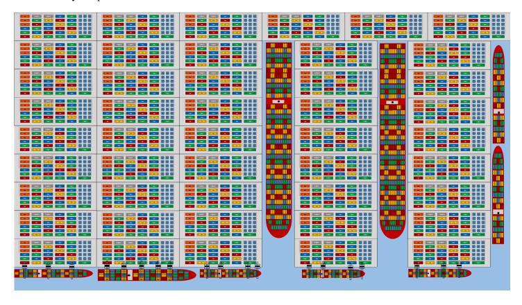
Many years ago, Amsterdam designed and built a berth where the ship could be worked from both port and starboard sides. unfortunately, the designers didn't anticipate the growth of vessel size. As ships got bigger, they could no longer fit into the berth and eventually, the terminal was closed down.
