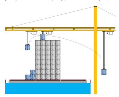
I think it is also safe to assume that by this stage, crane operations will be fully automated so the fact that the vessel is so much deeper will not cause the problems we see today because the crane operator is further and further away from the containers they are loading or discharging. This automation should speed up operations dramatically because it could apply dynamic calculations to determine the distance the next container to be loaded or discharged.
