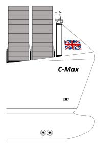
So far so good but this is where it starts to get trickier. Based on the above, the first thing to consider is pushing the vessel length up to 500m. Since the assumption is that these vessels will be autonomous, we can eliminate the need for a large accommodation. Instead, I have positioned a small bridge right at the forward end of the vessel for occasions where it may be that a pilot is required.
