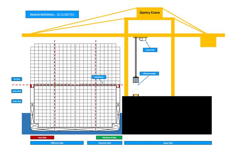
At present, the limitations on vessels are the outreach of the cranes, the height of the cranes and the draft of the terminal. The above profile would be the equivalent of todays 18,000 to 22,000 TEU vessels.
