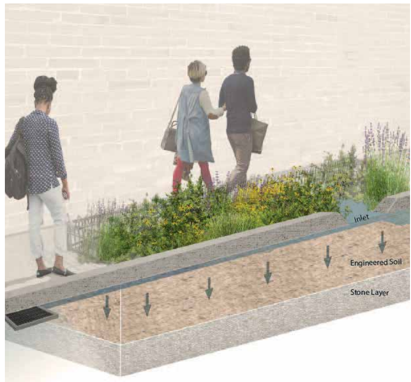
More than 30 bioswales that appear as miniature urban rain gardens were created by the City of New Haven to capture rainwater runoff and prevent flooding caused by heavy downpours and overtaxed storm drains. The city plans to install up to 300 more, 200 in the downtown area.
