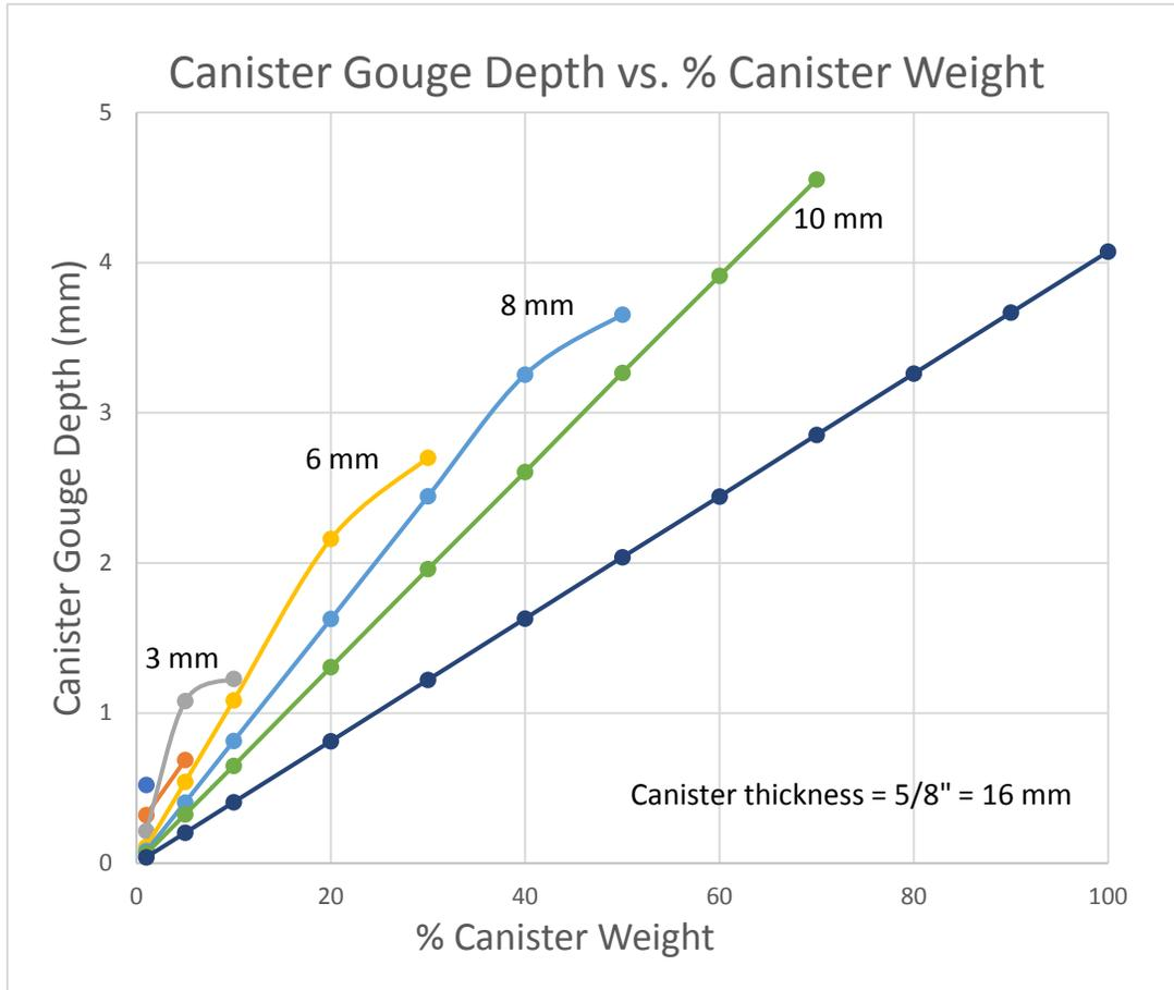
**Figure 4.** Calculated penetration depth of gouge as a function of load for different indenter diameter. The hardness number in Brinell scale for stainless steel 316 (BHN) is 217 kgf/mm<sup>2</sup>.
