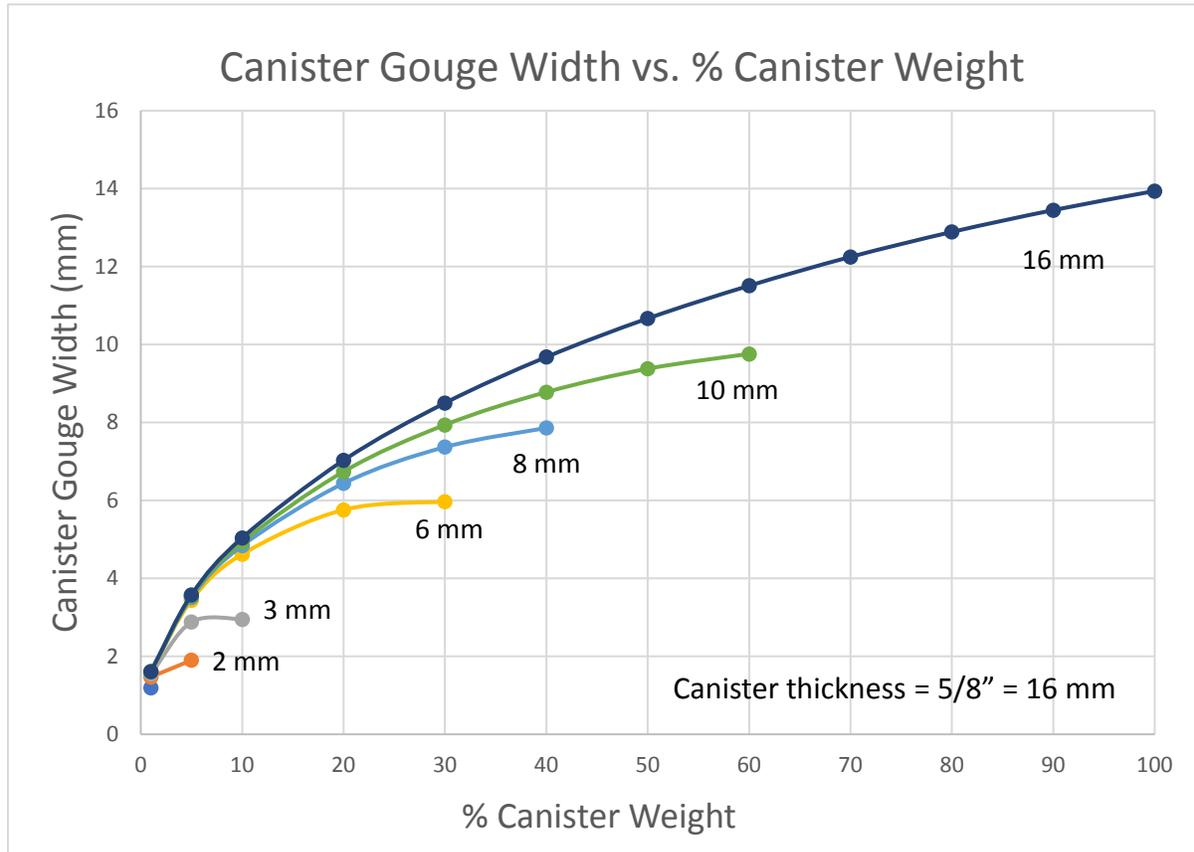
**Figure 3.** Calculated penetration width of gouge as a function of load for different indenter diameter. The hardness number in Brinell scale for stainless steel 316 (BHN) is 217 kgf/mm<sup>2</sup>. Saturated zone is eliminated.
