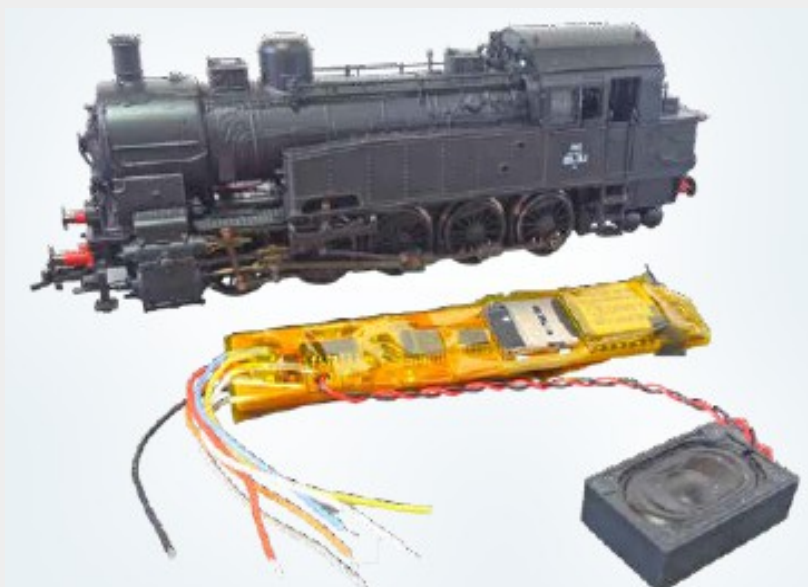
Photo 2. The LocoFi decoder is quite large: it will not fit in this O50 Fleischmann.
