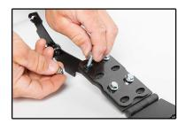
**Step #1:** Place throttle-MAXX gas pedal accessory on bottom side of gas pedal. Slide the four bolts face down through aligned factory holes and use 10mm wrench to tighten nuts.
