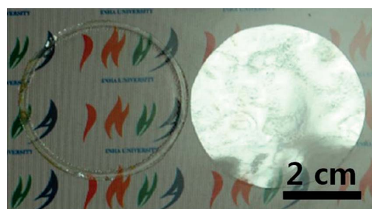
Fig. 5 Digital images of an AR film with N-ARS on both surface (left) and the reference flat film on the LCD monitor of a notebook computer.
