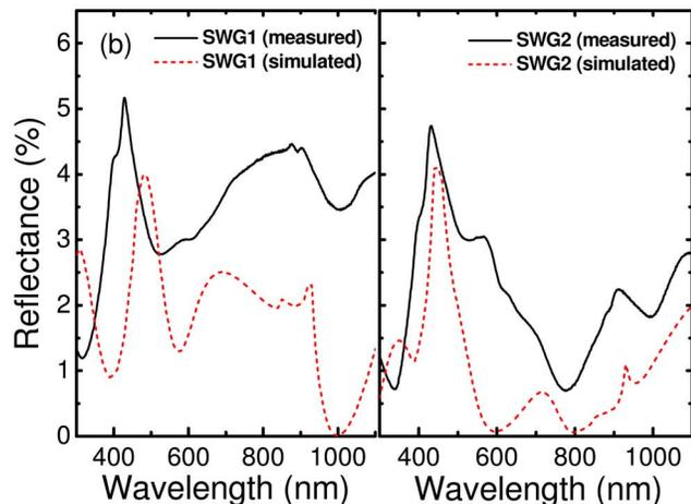
Fig. 4. (Color online) (a) Measured reflectance as a function of wavelength for the fabricated GaAs SWG1 and SWG2 structures. The measured and simulated reflectances of bulk GaAs were shown as a reference. The inset shows an SWG structure with conical profile used in this simulation. (b) Simulated reflectance spectra of the fabricated GaAs SWG1 and SWG2 structures were shown together with measured results.
