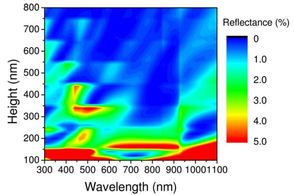
Fig. 5. (Color online) Contour plot of the variation of reflectance as a function of cone height and wavelength for a 300 nm period of the array.
