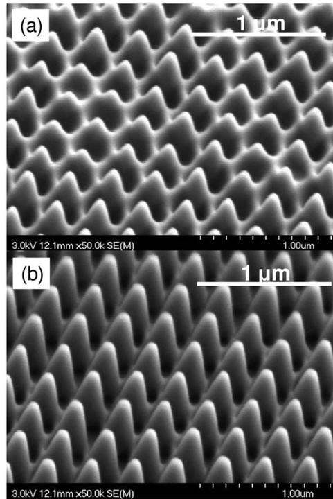
Fig. 3. SEM images of the fabricated GaAs SWG structures with different rf powers: (a) 150 W for 15 min (SWG1) and (b) 100 W for 12 min (SWG2).
