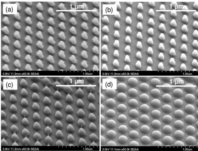
Fig. 2. SEM images of the PR patterns on GaAs substrate (a) before thermal reflow process and after thermal reflow treatments of (b) 160°C, (c) 180°C, and (d) 200°C for 40 s.
