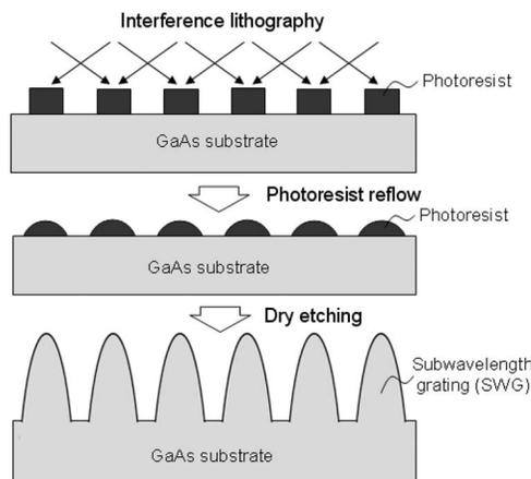
Fig. 1. Schematic illustration of the lens-like shape transfer procedures for the fabrication of the SWGs on GaAs.
