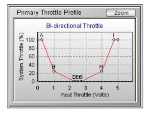
The curve plotted in this graph represents the way the controller will respond to the parameters that have been programmed into the software. As changes are made to the throttle parameters, the shape of the curve will change. For a larger view of the graph, click "Zoom" in the PC Probit II software.
