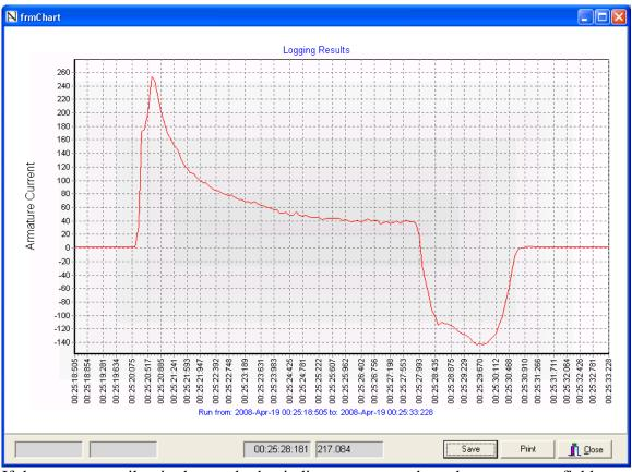
If there are any spikes in the graph, that indicates an area where the armature or field map variables will need to be adjusted.
