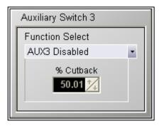
AUX3 Disabled Speed Limit 3 Input % Cutback when disabled, controller ignores this switch input forces controller into reduced speed mode 3 when active percentage of full speed utilized when Speed Limit 2 Input is activated "MOTOR SPEED SETUP" parameters:
