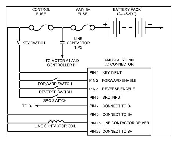
**Basic I/O Wiring (throttle not shown)**
