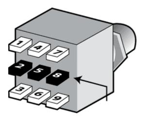
The pins on the switch must run left to right like this, so the top row of pins would be 1, 4, and 7.
