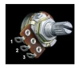
Pin Numbers for the pots. Snap the little metal tag off before trying to put it through the holes in the box.
