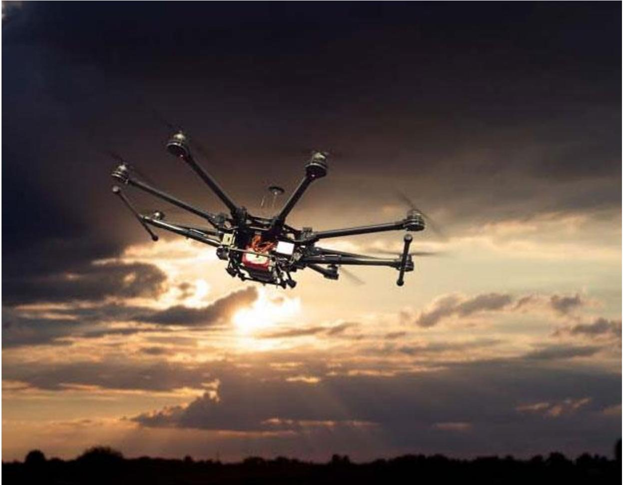
*Argus can photograph a large outdoor crime or accident scene utilizing AutoPilot in just minutes and then process all the images into a single orthomosaic photograph with GPS designations and then we can turn that into a 3D Model.*
