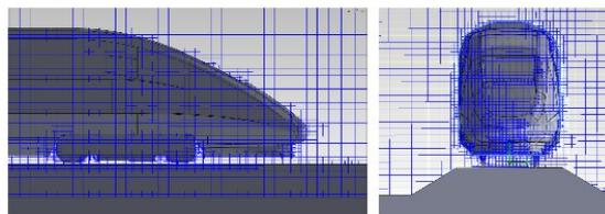
Fig. 3. Transverse and frontal views of the numerical discretization of the train.
