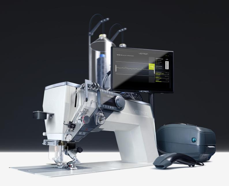
SIDE AIRBAG SEWING MACHINE FOR DOCUMENTED SEAMS, WITH TRIPLE TRANSPORT
