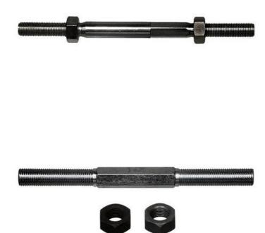
Above you will see the only two adjuster rods sold by MOOG for the Isuzu. The longer one on the top ES3089S measures 8.42" from end to end and is listed for 2WD Isuzu Pickup Trucks. The shorter one on the bottom ES3090S measures 6.63" from end to end and is listed for Amigo 1988-1994, 4WD pickup 1988-1995, Rodeo 1991-1995, Trooper 1987-1991.
