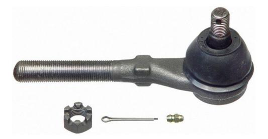
Above is Moog ES3369T and ES3370T which upgrades the rod thread to 18mm but keeps the same stud thread and taper so it will bolt up to the stock knuckle.
