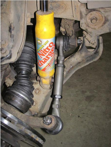
Here is the finished installation on a 1990 Trooper. Remember to set the length of the tie rods as best you can to match the old ones you take off. This will get you close enough to drive to the alignment shop. If the caster and camber were good before then all you will
