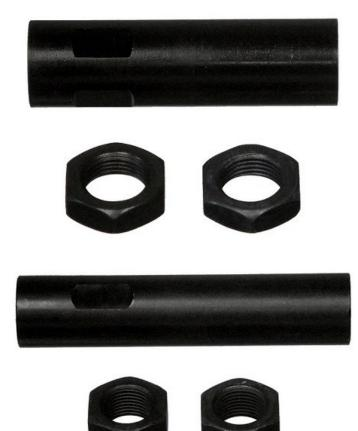
These sleeves are what makes these ordinary parts so much stronger than the stock ones. These solid sleeves are available off the shelf from MOOG one is ES3201S which measures out at 3.35" end to end and will cover Amigo 1988-1994, 4WD pickup 1988-1995, Rodeo 1991-1995, Trooper 1987-1991. All of these application will require cutting off 7/8" from the male threads on the tie rod end to make them shorter so they don't bottom out against each other in the sleeve and allow for proper alignment.
