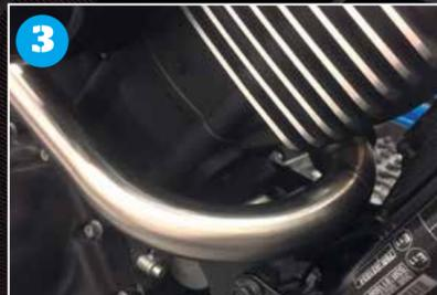
**Step 3** Reaching the front cylinder is straight forward, so Geoff bends the first primary so it runs under the air filter whilst also allowing access to the oil filler cap, and keeping in mind the need for ground clearance.
