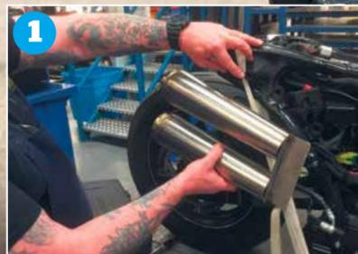
**Step 1** Starting with a pair of GFMoto S1000RR end cans, fabricator Geoff Rayner works out where to put the collector – the part that takes converts the two pipes into one, then back into the two end cans.
