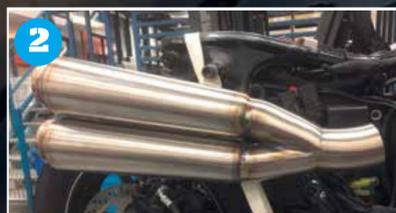
**Step 2** Geoff then expertly tig welds the collector unit then works out how much pipe he needs to reach the cylinders. As weight is not as much of a consideration, he's working in T304 stainless steel.
