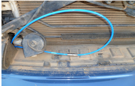
Figure 9 – completed loop in grill area. Arrow points to line that feeds into the air-bag
