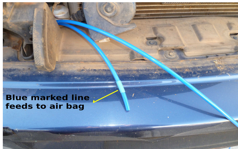
Figure 8 – feed in the lines to wheel-well area
