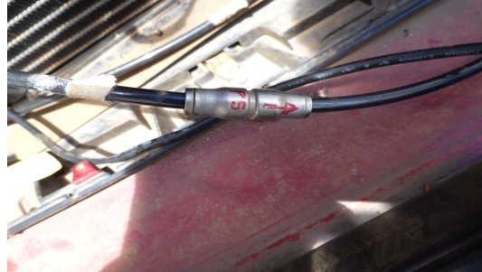
Figure 9 – completed loop in grill area. Arrow points to line that feeds into the air-bag
