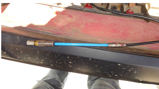
Figure 11: Shraeder valve + short line attached to the circuit.
