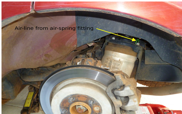
Figure 7 – location of connector on rear air-spring
