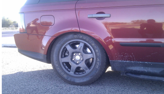
Figure 5: Rear of RRS down on bump-stops- a 265/60R18 tyre
