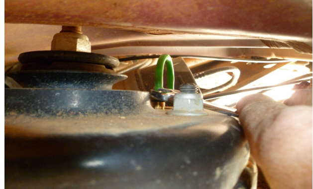
Figure 7 – location of connector on rear air-spring
