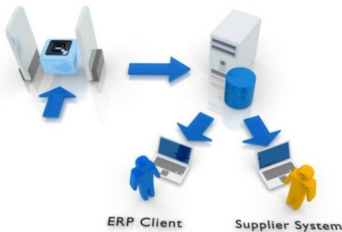
First and foremost RFID is a system. An RFID system is a hands free or wireless way of reading data (usually in the form of an ID number), from a distance, using a specific radio frequency. An RFID system includes: an RFID tag, followed by a reading device, which has radio-enabled communication with the tag and a software component that can interpret the data read from the tag. As mentioned above, there are several
