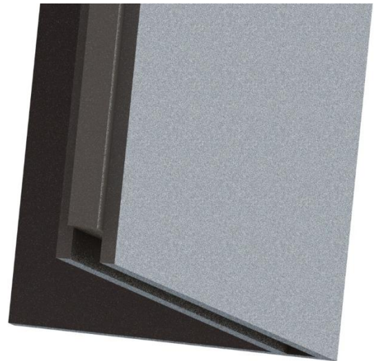
Figure 11 & 12. The base has an extrusion along the sides while the cover has a slot of equal dimensions. The base also features a slot in the back while the cover has an extrusion along the back of equal dimension. Since the case is made of ABS Plastic, the cover will slide onto the base with force and will remain during the Inspire's flight.
