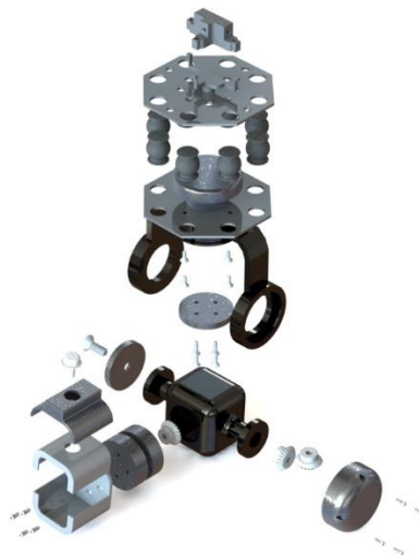
Figure 16. Exploded view of Gimbal.
