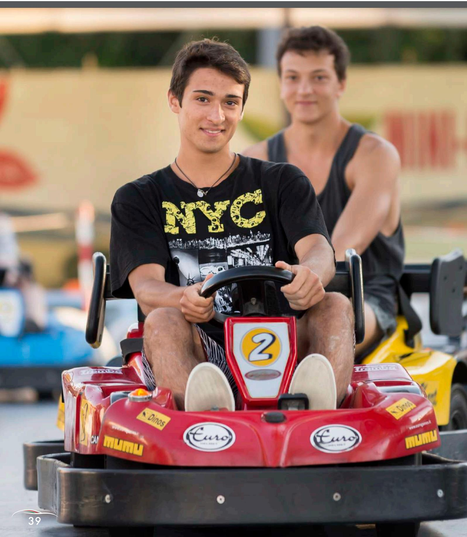
Equipped with a powerful 780W brushed motor, Eurogames battery operated Go Karts are specially designed for amusement venues like Family Fun Centers and Amusement Parks. Featuring accelerator and brake pedals, our one-seater or two-seater Go Karts are supplied with disc brakes and can do up to 12 mph (20 km/h) with 1 or 2 speeds.
