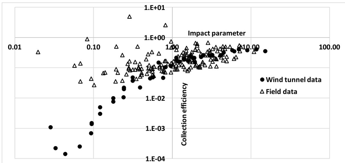
Fig. 6. Comparison of the relationship between measured collection efficiency and impact parameter for wind tunnel data (using Eqn 6), and that estimated for field data using Eqn (4).
