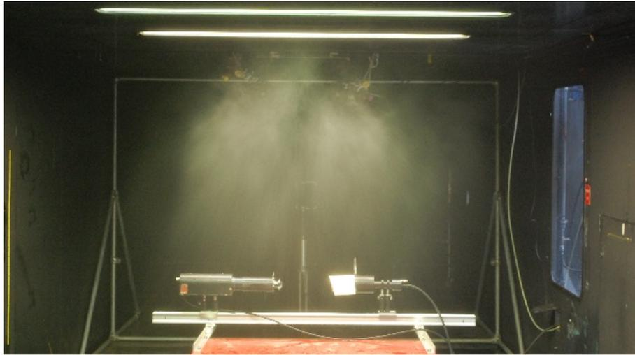
Fig. 1. Nozzle layout and instrumentation for droplet size measurements: view from the end of the tunnel looking upwind into the spray cloud with the Visisizer mounted on a moveable platform.
