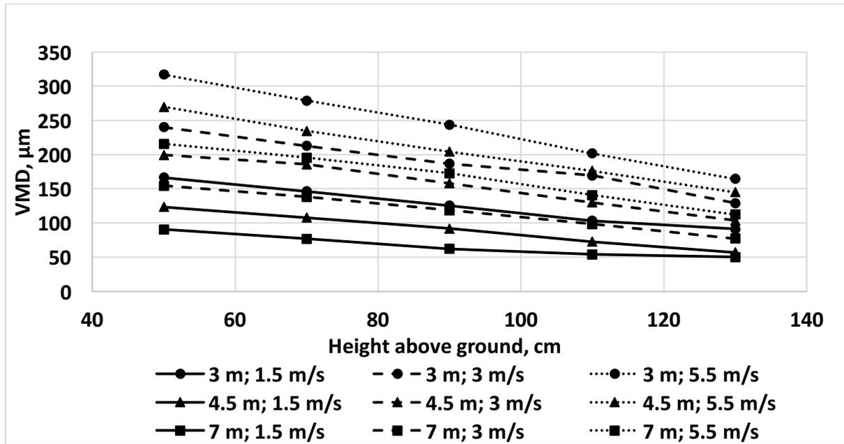
Fig. 4. Variation of mean VMD (averaged over three lateral values) of spray with distance, height and wind speed.
