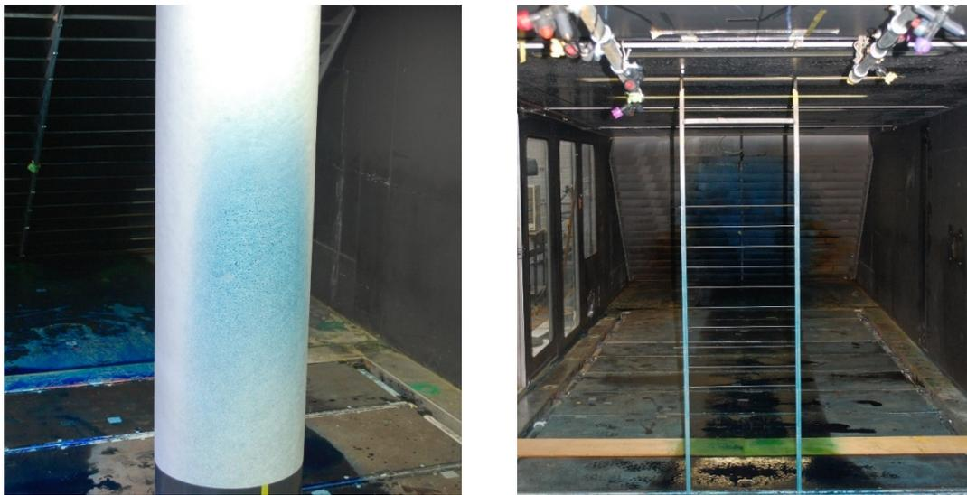
Fig. 2. Tyvek® sheet wrapped around the 0.4 m cylinder (left) and set of lines for collecting airborne spray (right).
