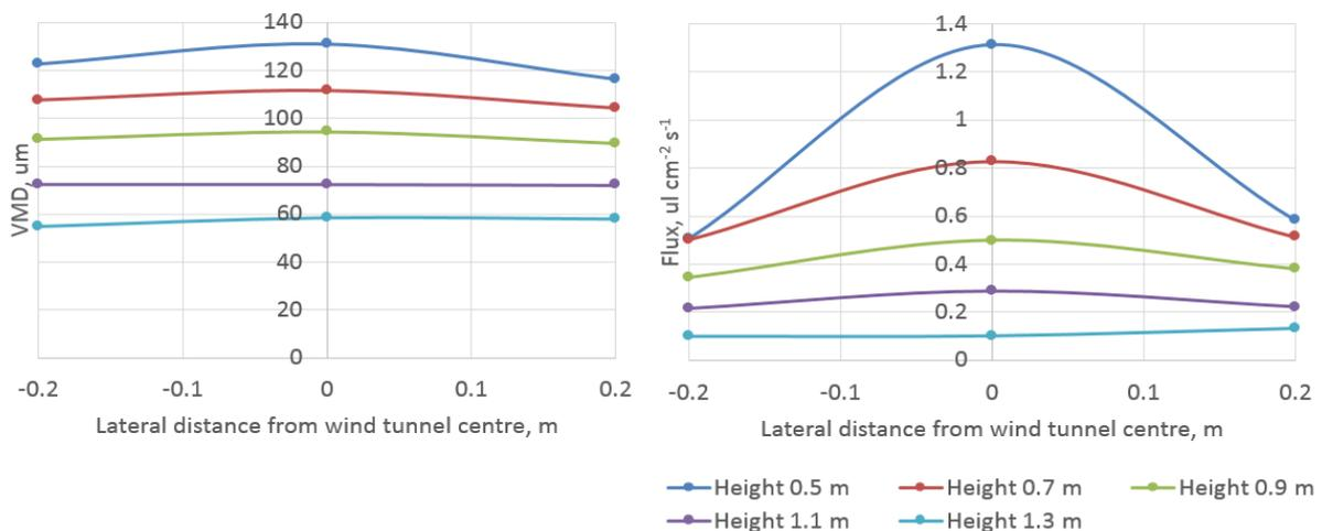
Fig. 3. Variation of VMD (left) and flux (right) with lateral position in the wind tunnel, 4.5 m downwind and with a wind speed of  $1.5 \text{ m s}^{-1}$ .
