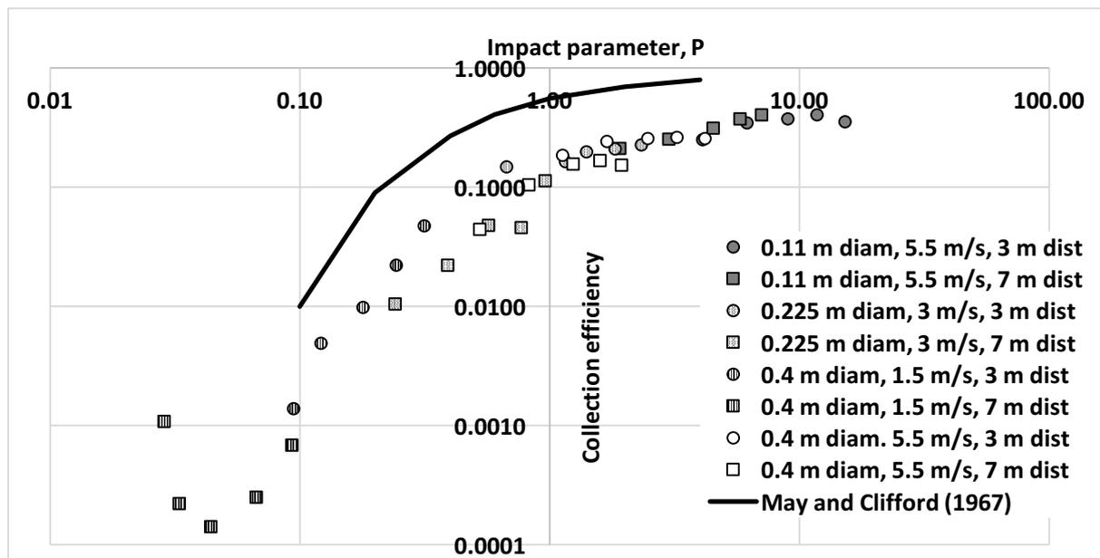
Fig. 5. The relationship between impact parameter and collection efficiency for a range of cylinder diameters, wind speeds and distances downwind.
