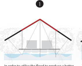
In order to utilise the flood to produce a better design, the structure allows the flood to push the platform vertically upwards. It does this through the use plastic barrels as the predominant substructure, because it cannot be immeresed in water and so must fully stay afloat, therefore continously pushing the platform above it.
