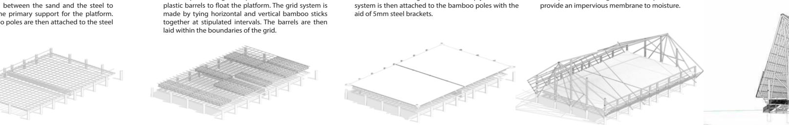
Finally, the roof is made by interlocking bamboo poles cut in half. After which it is attached to the previously pegged bamboo posts/columns and rafters.
