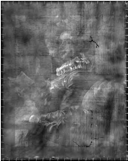
19. X-radiograph of Young girl reading obtained using Carestream System, 40KV.
