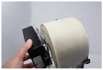
ATTENTION: Before tilting the black box, move the used media roll manually back and forth to UNLOCK the direct drive.
