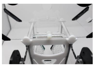
After setting the position of the top module, ensure front and back screws (back screw shown) are tight enough to restrict movement of the top module
