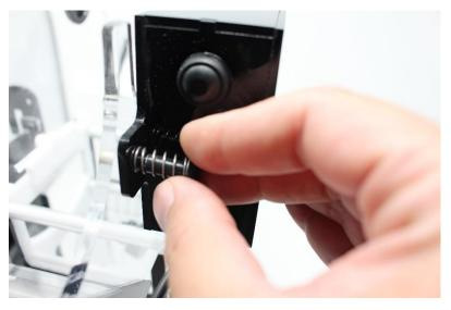
Set the long black screw with the **spring** to secure the black box with the top unit. Turn the screw clockwise and make sure the screw doesn't protrude on the other side.
