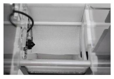
Pass the media over the top rod and under the lower rod as shown
