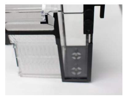
The Vortex Generating Bypass Controllers are positioned at the bottom of the overflow section of the unit.
