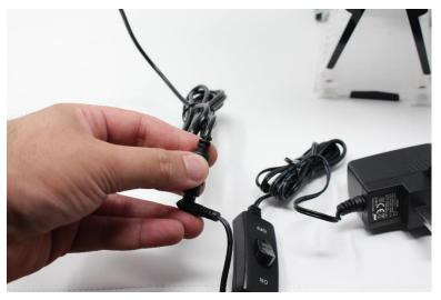
After installation, use the power supply provided and connect it with the cable from the black box with.
