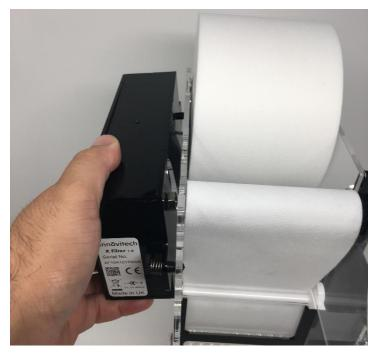
By sliding the black box outwards, clearance will be created from the direct drive to let the spool sit into place
