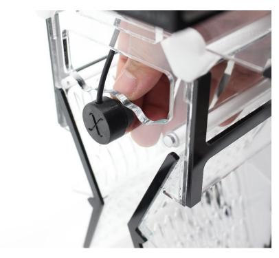
Secure the sensor with the plastic nut provided and make sure the sensor has a good seal with the bottom (main) unit. (The sensor has a gasket set on the base of the sensor).
