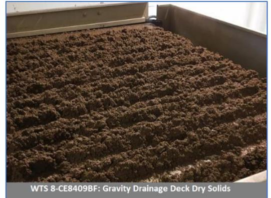
WTS 8-CE8409BF: Gravity Drainage Deck Dry Solids
