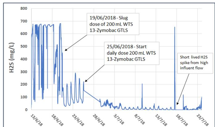
Figure 1: H<sub>2</sub>S levels monitored from the balance tank hatch before and during the WTS 13-Zymobac GTLS treatment.
