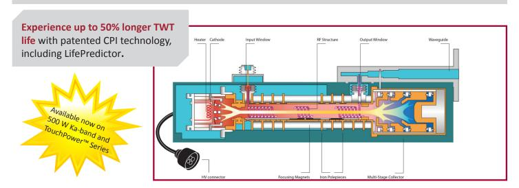
CPI's LIFEEXTENDER is new, patented technology which is a leap forward over other methods introduced to the satcom amplifier market to increase traveling wave tube (TWT) life. CPI's dynamic LIFEEXTENDER is the only method where the life of the TWT is extended by preserving the active coating on the cathode surface.
