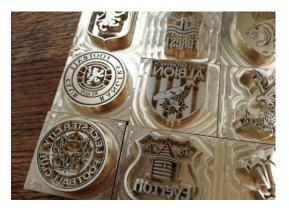
Our Dies are made from 1/4" thick brass and deeply etched.
