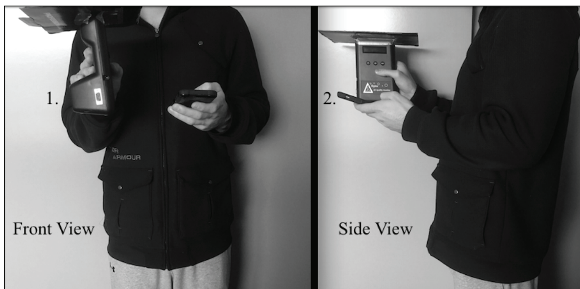
Figure 2: Instruments and orientation during data collection (1. Dylos 1700 Optical Particulate Matter Sensor, 2. Motion X GPS iPhone App and iPhone Voice Recorder)
