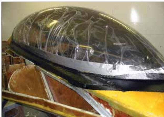
Canopy prior to being cut off. Yep, it's bedded in carbon fiber. Most of the airplane is constructed with E-Z Pox.
