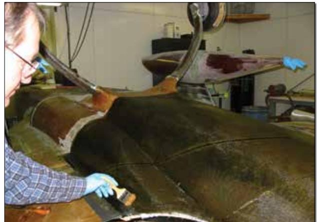
Robert doing a layup on the bottom of the Jet Eze's carbon fiber cowling.
