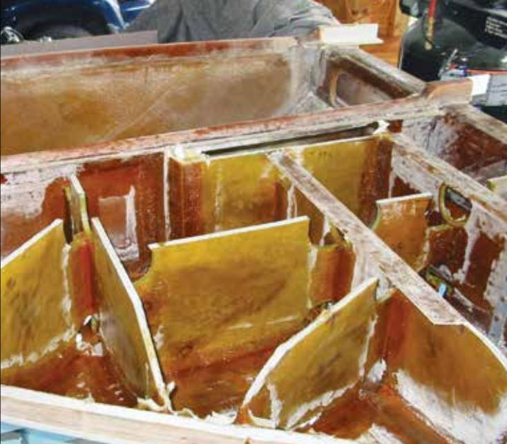
Internal structure of the left strake. I built two sub spars to carry the load of the fuel and baggage pods.
